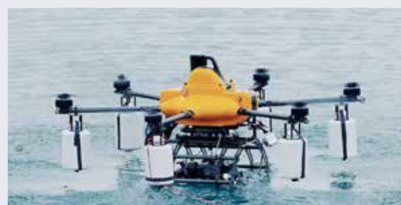
“Amphibious drone” to be used for underwater inspection work, etc.
