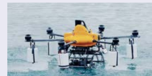
“Amphibious drone” to be used for underwater inspection work, etc.
