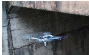
▲A drone active in bridge inspection
