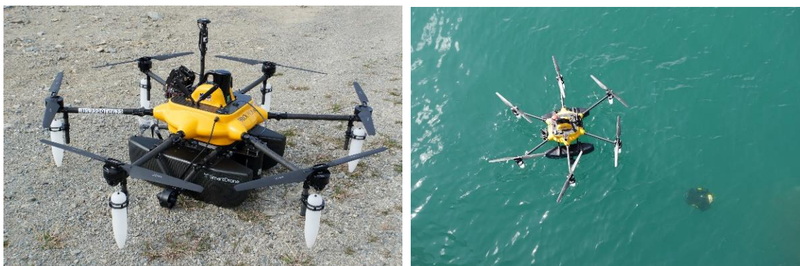
Fig. 19 Base unit (left) The sub-unit separates from the base unit and dives underwater (right)
